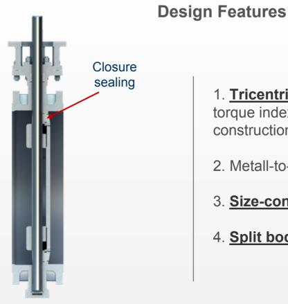
1. Tricentric construction ensures lower torque index in comparison with customary constructions.
